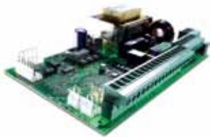
JE275 bollard control board it controls 1 J355 M30-P1 bollard
